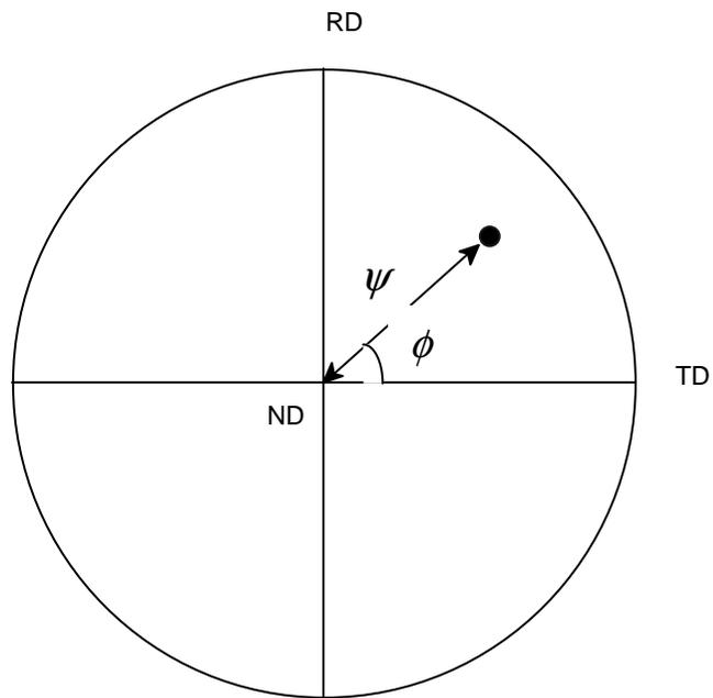
Specimen coordinate system on a stereographic projection (often used for rolled specimens)
