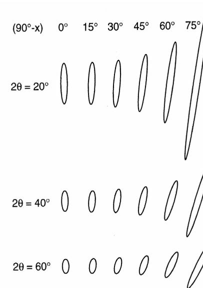
Change in shape and orientation of the irradiated spot on the sample surface for different sample inclinations as a function of tilt angle and Bragg angle (Bunge).
