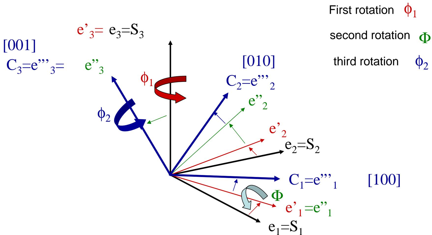
First rotation  $\phi_1$  around  $S_3$  transforms  $S_1$  and  $S_2$  axis in the new axes  $X_1'$  and  $X_2'$ . The second rotation  $\Phi$  around  $X_1'$  axis has to align the  $S_3$  axis to the  $C_3$  axis and transforms  $X_2'$  to  $X_2''$ . The third rotation  $\phi_2$  around  $C_3$  aligns  $X_1'$  to  $C_1$  as well as  $X_2''$  to  $C_2$ .
