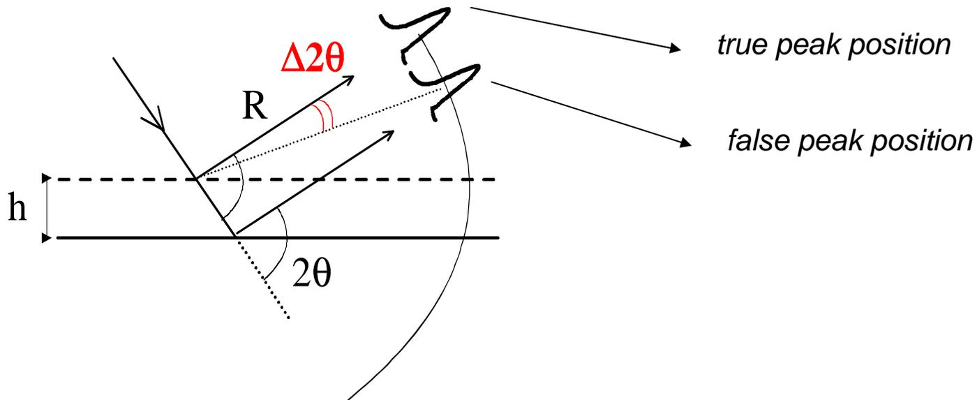
The error due to the sample displacement depend on  $2\theta$  angles:
