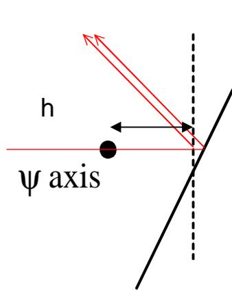
Displacement in the psi geometry:
