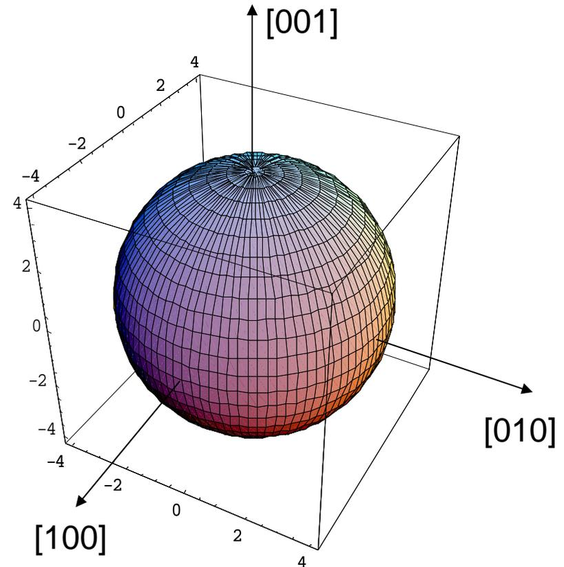
Young's modulus can be represented by means of a spherical polar diagram, that is, with a surface generated by a vector whose length is proportional to the value of Young's modulus in the direction pointed by the vector itself.
