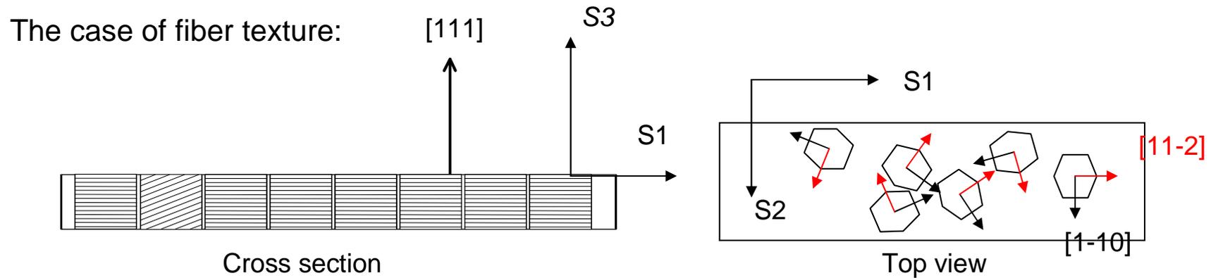
Consider a thin film (700 nm thick) with a columnar microstructure in which the (111) planes are parallel to the surface, but randomly distributed in the plane of the surface → this is the (111) fiber texture
