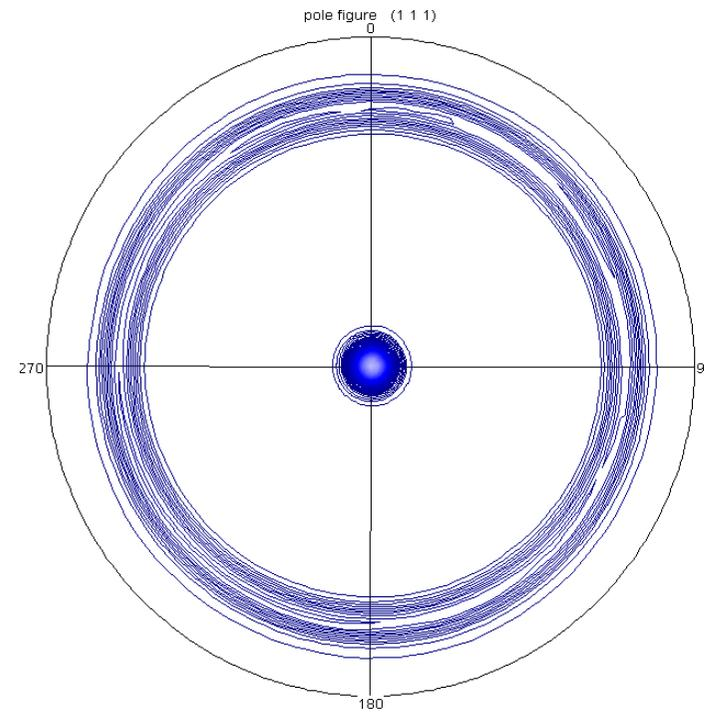
Different view of the {111} pole figure on a gold thin film, TEM micrograph
