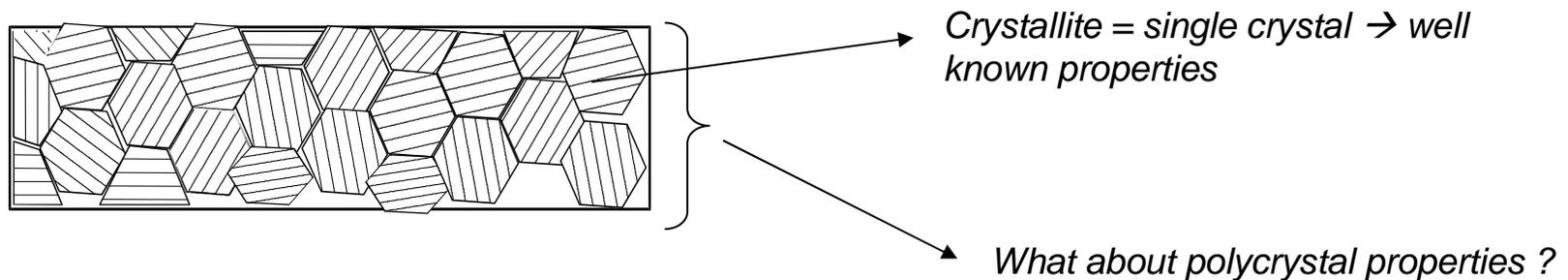
In a polycrystalline material, the strains differ between grains and all grains interact with each other due to the incompatibility of these different strains. As a consequence, the average stresses in each grain also differ.
