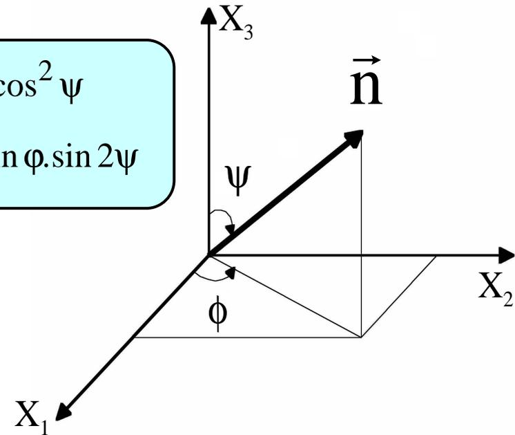
The strain in the direction  $n$  can be related to the lattice spacing:
