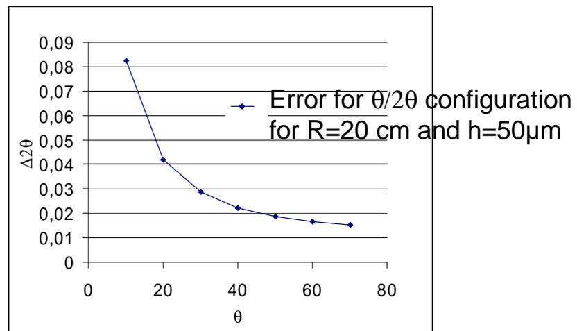
Moreover, if the specimen is displaced from the center of the goniometer, the error in 2theta angles will depend on the psi angles.
