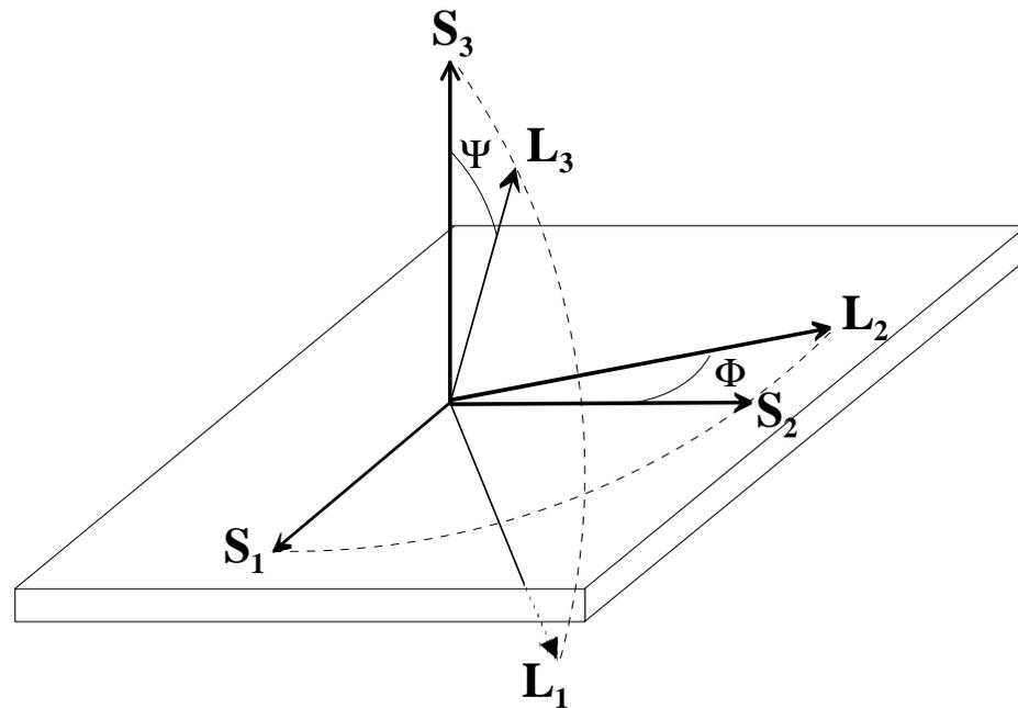
*Orientation of the laboratory system relative to the specimen system*
